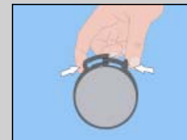
2. Engage the first few teeth by hand to hold the clip in place.
