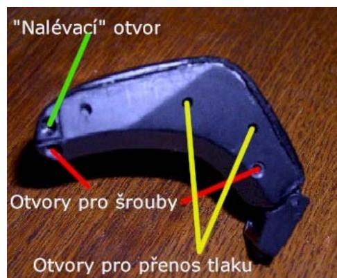
**Green** - Filling hole. Through this hole you can refill oil (if it is not blocked inside by glue) This hole is covered by a screw with Oring.
