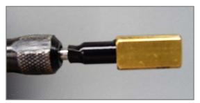
If you are doing a *Mistral* HP seat you will need to put a couple of turns of tape around the mandrel to make the seat fit tightly inside it.
