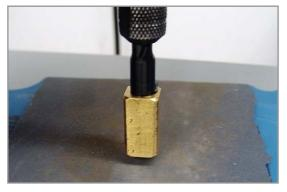
If you are doing an *Aqua-Master* seat you can simply chuck it right into the rotary tool.
